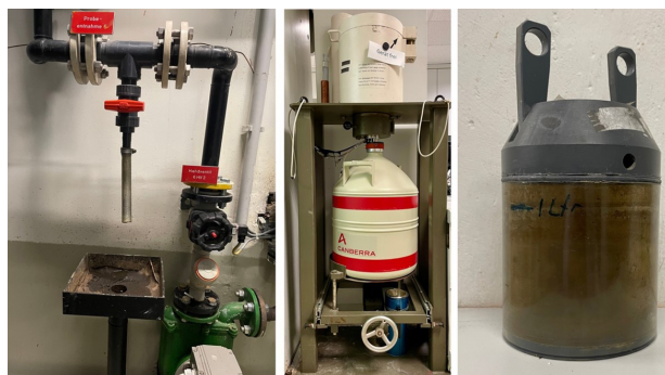
Figure 5: Sampling point (left), sample measuring station with HPGe detector (centre) and Marinelli vessel (right)
