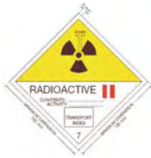
Figure 3: Category II Yellow Label. The background colour of the upper half of the label shall be yellow and the lower half white, the colour of the trefoil and the printing shall be black, and the colour of the category bars shall be red (1).
