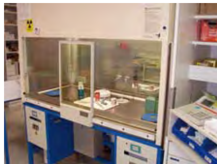
Figure 1: Laminar flow unit for preparation of ^{99m}\text{Tc} radiopharmaceuticals
