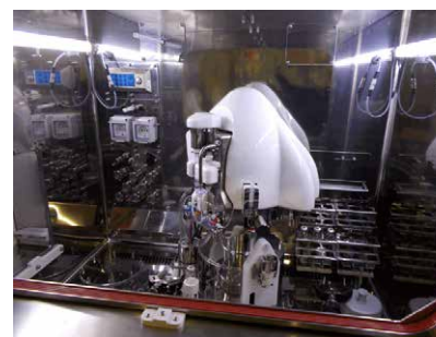
Figure 6: Automatic dispenser for PET tracers
