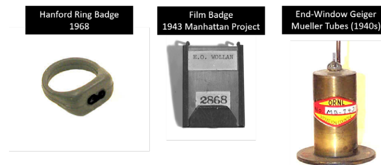
Figure 2: Left: The Hanford ring badge, used to determine exposures to the hands of workers manipulating radioactive sources. Centre: Film badge dosimeter from the Manhattan project. Right: End-window Geiger-Müller tube for measurement of radioactivity
